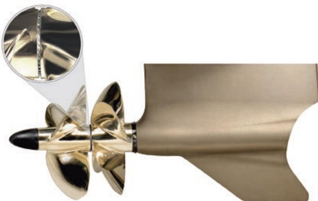
**The line cutter** is mounted to the rear propeller which creates a very efficient rotating cutting action. It is easy to install using the existing locking bolts and does not increase drag or fuel consumption.
